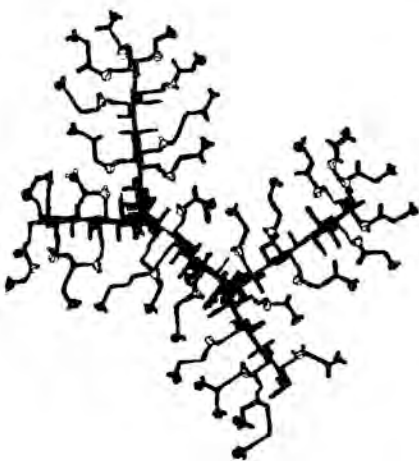
“Stem” development, Caen Herouville. Shadrach Woods, architect, 1961. Linear organization of activities and the proposed grouping of cells around the linear center.
